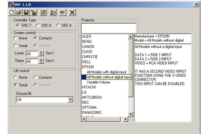
\* There are only 2 x RS232 ports so if you use a lift the closed contact should be used for the screen
