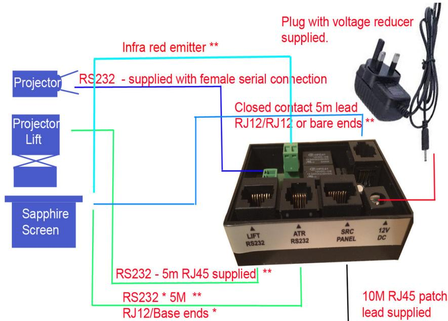
The control panel is powered from the breakout box via the standard 10M Cat 5 cable supplied.
