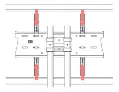
Gently lower the screen until the arms are securely hanging on top of the back plate. Once centered, adjust the level of the screen with the two top Screws on the mount arms. Once leveled secure the screen by tightening the bottom two screws.
