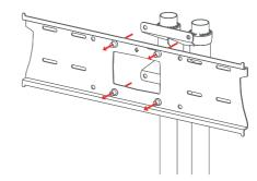
Once placed over columns and at the desired height, tighten the two grub screws to secure into place. Tighten up the base grub screws to secure.
