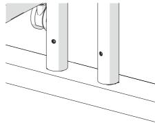
All columns have a half-moon notch at one end and 2 of the columns will have holes at 75mm from one end (these will typically be the longer pair of columns). Place the 2 columns with holes over the crocodile lugs on the base.
