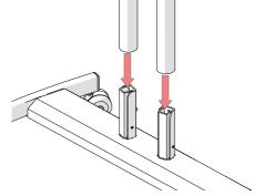
Turn the base upside down and push each castor until it clicks into place. Please ensure that the castors with brakes are located at the front. Place base on the floor and apply brakes on front wheels by pressing brake lever down.
