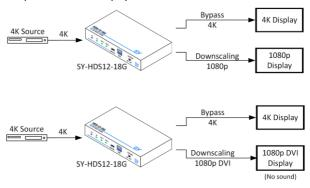
Each output can independently Auto-downscale from 4K to 1080p, depending on the capability of the display device. This ensures optimal use of mixed capability displays.
