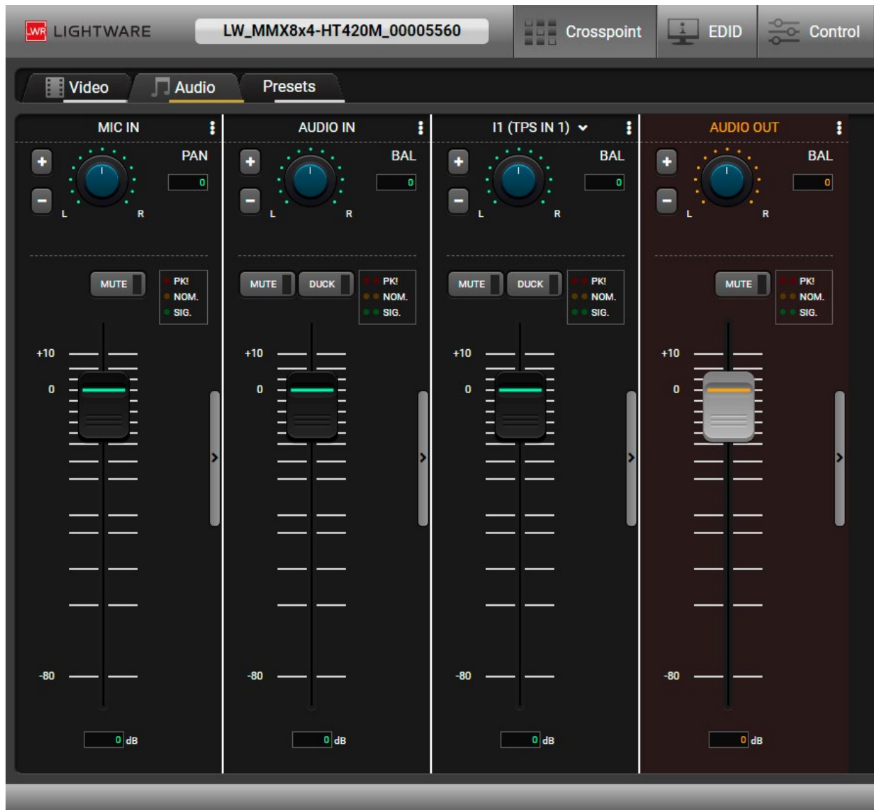
Audio tab in the Crosspoint menu – Basic settings can be seen on the default view
